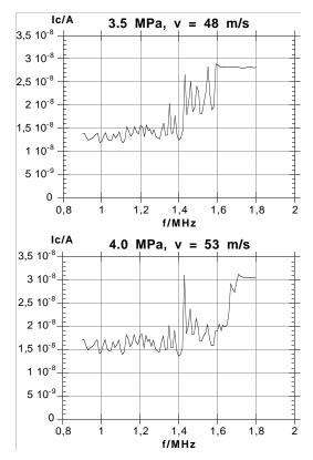
Figure 7. Charging current measured at two jet velocities when the stimulation frequency was varid between 0.9 - 1.8 MHz.
