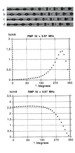
Figure 8. Results from the measurement of the width of the forbidden region for a drop formation frequency of 0.97 MHz. The satellite cut-off occurs after the main drop cut-off. The drop formation is shown above for a) 0, b) 90, c) 180 and d) 270 degrees phase with respect to the main drop cut-off.
