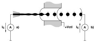
Figure 3. Charging current measurement. a) Through the ink ground terminal. b) Through discharging of the charged drop.
