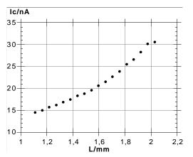
Figure 6. Charging current vs. the distance to the PODF for a 9.5  $\mu$ m jet traveling at a velocity of 53 m/s. The stimulation frequency was set at 1.0 MHz and the charging voltage was 40 V.
