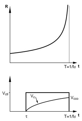
Figure 5. Principle for the applying of the region measurement pulse (RMP). The drop is charged during the on-time of the pulse.
