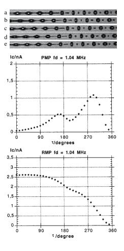
Figure 9. Results from the measurement of the width of the forbidden region for a drop formation frequency of 1.04 MHz. The satellite cut-off occurs before the main drop cut-off. The drop formation is shown above for a) 0, b) 90, c) 180, d) 225 and e) 270 degrees phase with respect to the main drop cut-off.
